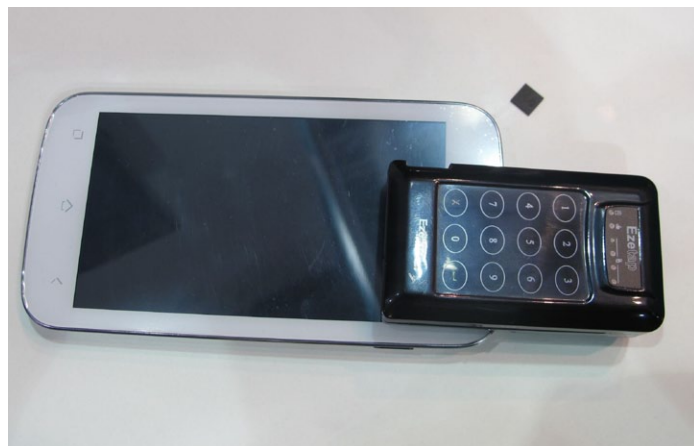
Built around Maxim Integrated's USIP-L (the small black chip), the Ezetap MPOS unit connects to smartphones either through their audio-jack, USB or Bluetooth.
