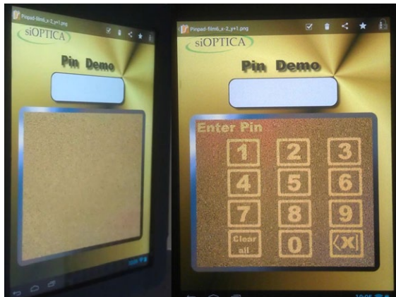
siOPTICA' siOSwitch combines a passive polymer display overlay and special software.
