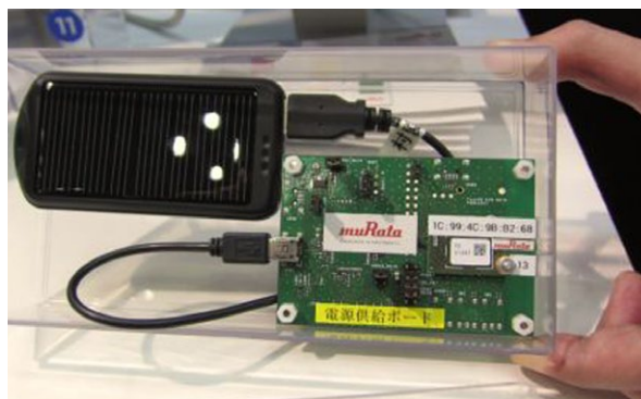
A WiFi-based mesh network solution tied to a solar-powered power supply.
