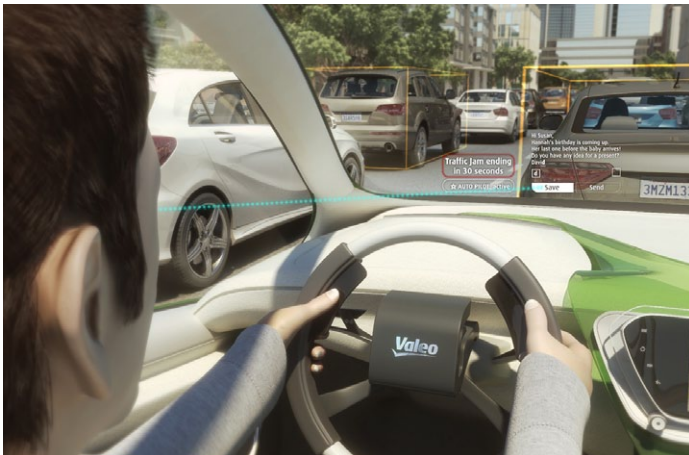
A potential eye tracking application: messages appear in the head-up display; the driver decides with a glimpse how to handle them.
