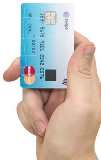
The Zwipe card runs its fingerprint authentication process battery-less.
