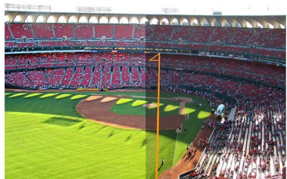
Fig. 7: Effects of the local area brightness boost algorithm.
