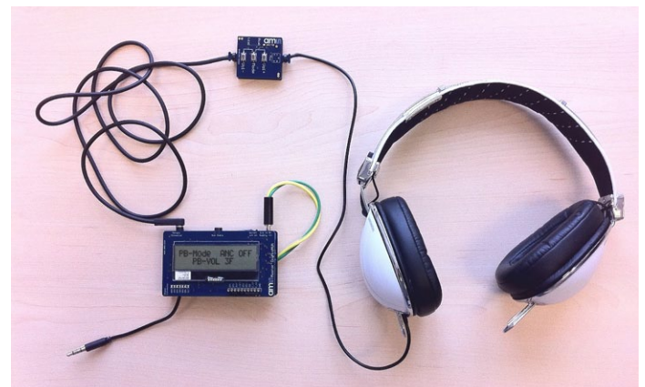
Fig. 2: The ams demonstration system, showing the master board (bottom), the peripheral circuit (top) with Volume Up, Mode and Volume Down buttons, and a headphone set.
