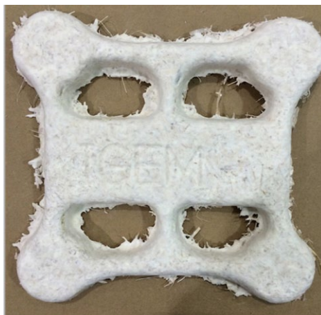
The bio-drone's chassis, made of mycelium, the vegetative part of a fungus, was modelled and 3D-designed by a team of students for the 2014 iGEM design contest and produced by Ecovative Design. Source: iGEM.org
