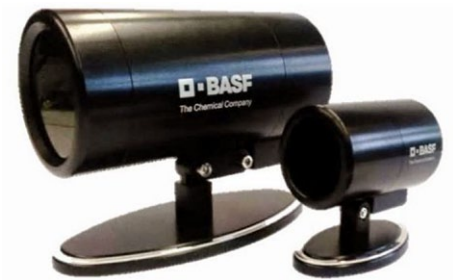
Prototype 2:0 cameras for position and color detection. Source: BASF
