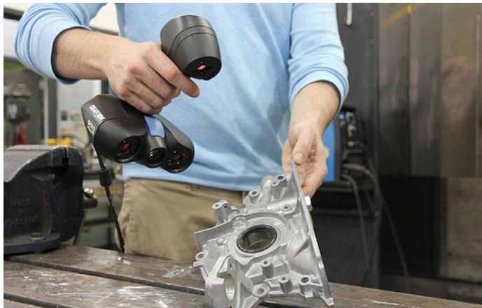
Creaform's Go!SCAN 3D handheld white-light 3D scanner.
