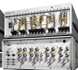
Keysight E6640B EXM wireless test set with V9080/82B LTE FDD/TDD measurement applications and N7624/25B Signal Studio software for LTE-Advanced/LTE FDD/TDD
