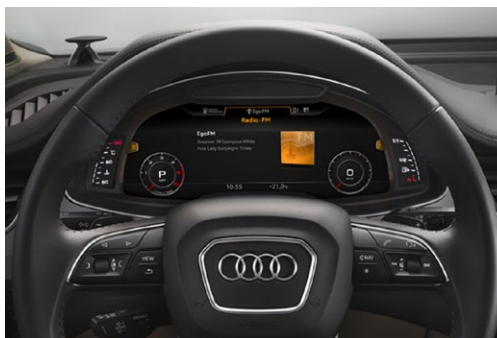
Nvidia powered virtual dashboard instruments
