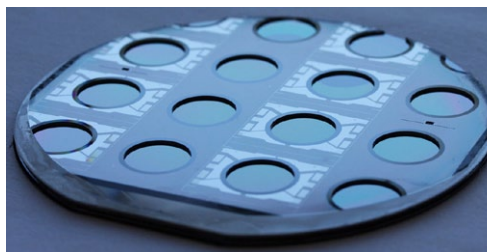
Mirror structures for a piezo-actuated Fabry-Perot. The optical apertures (round parts are 15.5 mm in diameter)
