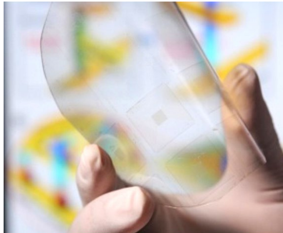
An array of piezotronic transistors making up taxels capable of converting mechanical motion directly into electronic controlling signals: Source Georgia Tech.
