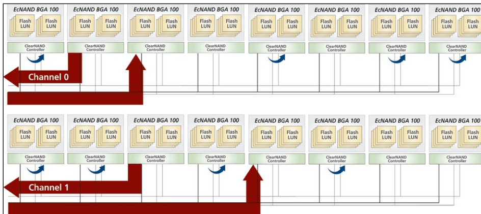
Figure 7: Copyback using enhanced ClearNAND flash
