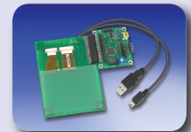
Projected Capacitive Development Kit - DM160211
