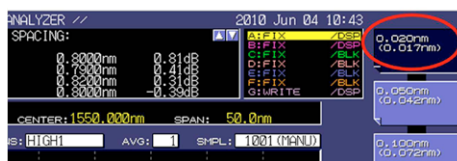
Figure 3: At 1550nm, the OSA has a stored value for the effective resolution of 17 pm, i.e. higher resolution than the selected 20pm
