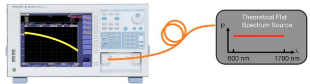
Figure 4: The recorded spectrum of a perfectly flat spectrum is dropping towards longer wavelengths
