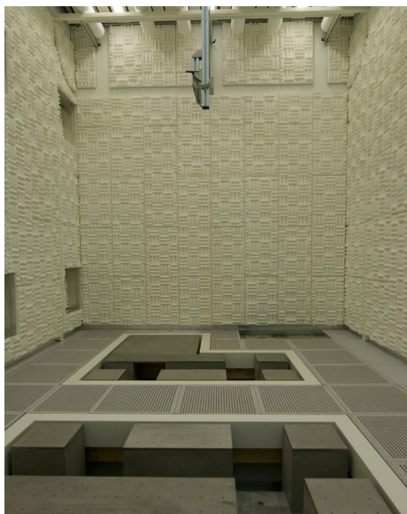
One of the noise-free labs in the basement. All feature vibration levels below 500nm/s and active electromagnetic fields compensation below 5nT AC.
