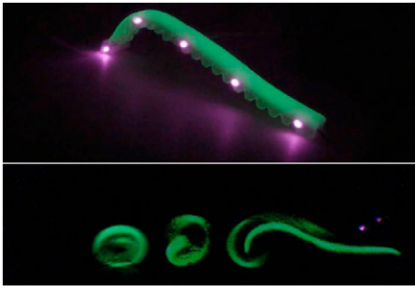
The caterpillar soft-robot from the Tufts Biomimetic Devices Laboratory is capable of crawling but can also jump into ballistic rolling.
