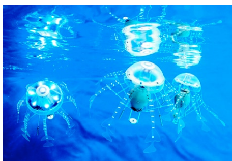
The AquaJelly's LEDs and light sensors enable the robot to communicate with others and emulate a swarming behaviour.
