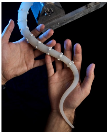
This manipulator arm directly inspired from the octopus' tentacles boasts infinite degrees of freedom. Source photographer "Massimo Brega - The Lighthouse".
